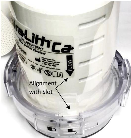
**Figure 1:** Place the cartridge into lid with the FLOW arrow aligned with one of the SLOTS in the lid/lock ring assembly
