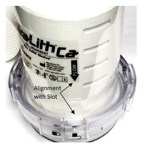
**Figure 1:** Place the cartridge into lid with the FLOW arrow aligned with one of the SLOTS in the lid/lock ring assembly
